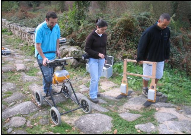
Figure 3. Acquisition tasks with the 200 MHz antenna.
