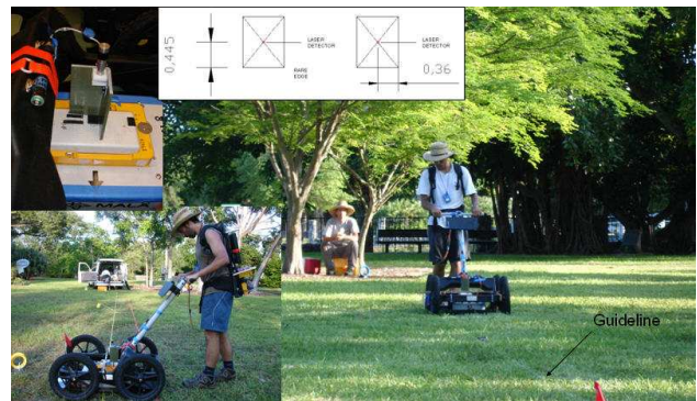
Figure 3. Methodology used with the standard GPR equipment: strings as guidelines for navigation, measurement tapes to place every profile and spray marks to help the operator to start and end each profile with better than 5 cm precision.
