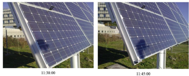
Fig. 5 Shadow caused by the anemometer
